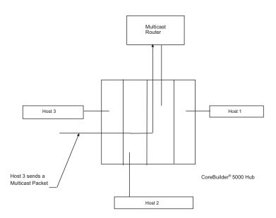
Figure 5-3 Multicast Packet Path after Snooping
